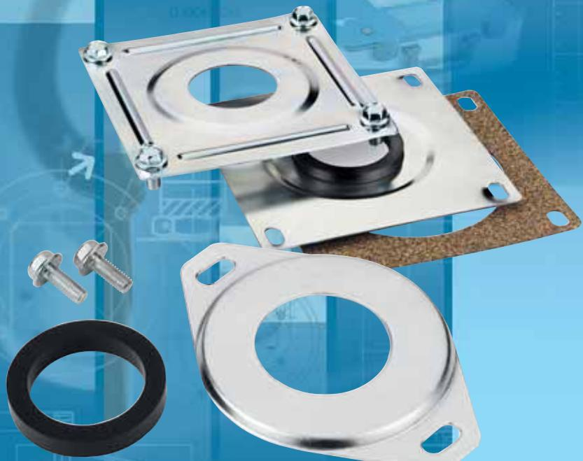
FT flanges make it possible to fix suction and return lines on the reservoir cover. Fitting a flexible insert allows separation of pipes. Both rigid pipes and flexible hoses can be separated from the reservoir walls, absorbing vibration and reducing plant noise emissions.
