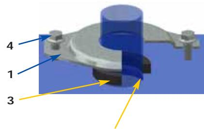
Drill the panel max 2 mm more than the pipe Ø
